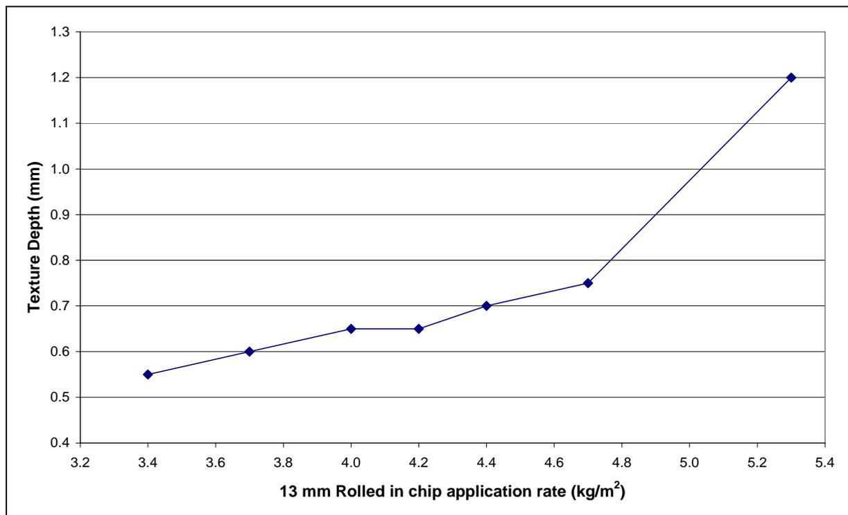
Figure 7. Comparison between rolled in chips application rate and surface texture.
