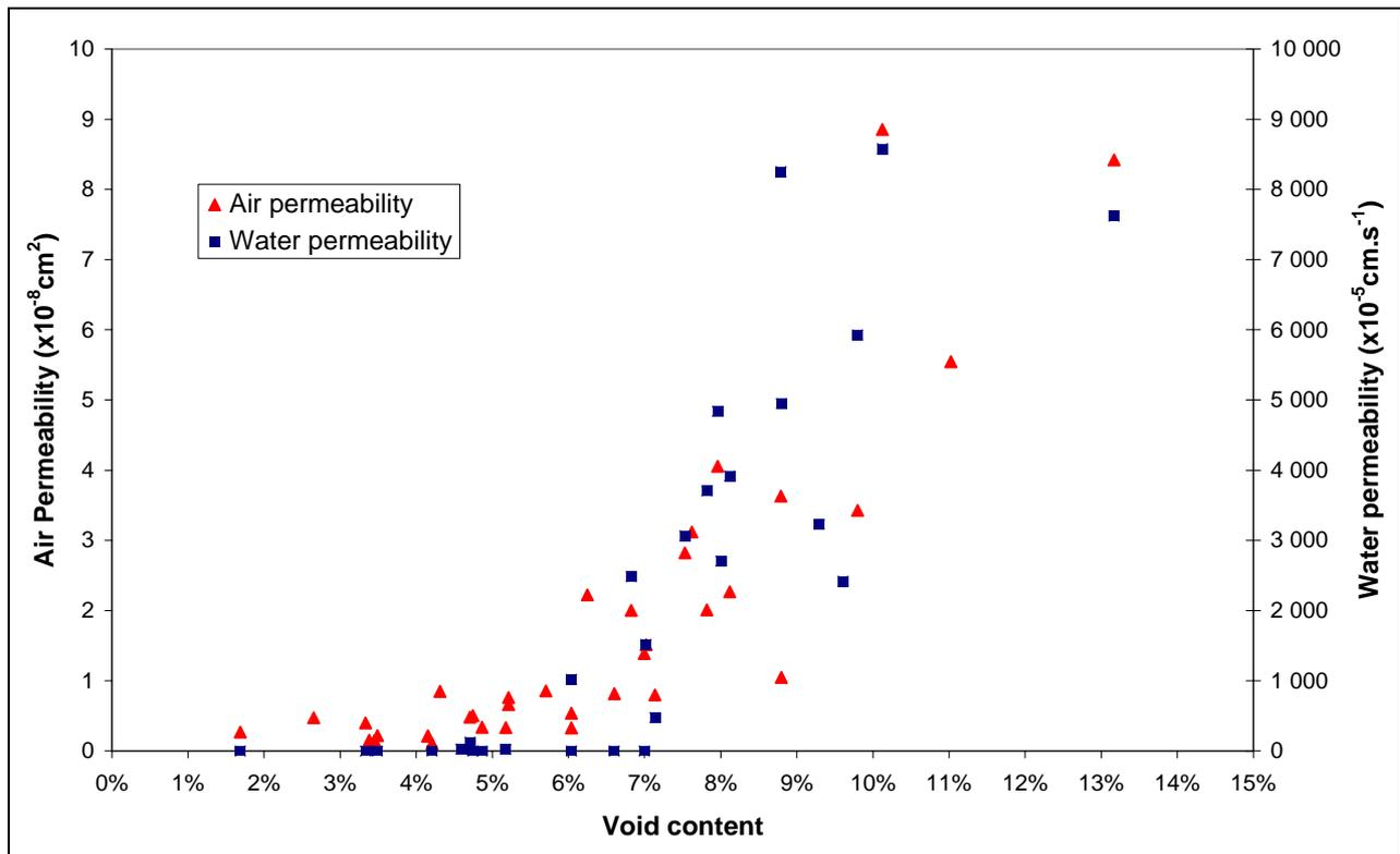
Figure 4. Medium continuously graded asphalt permeability test results.
