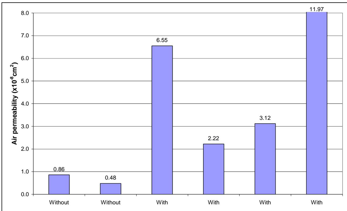
Figure 3. Comparison between air permeability of cores (medium continuously graded) with and without rolled in chips.
