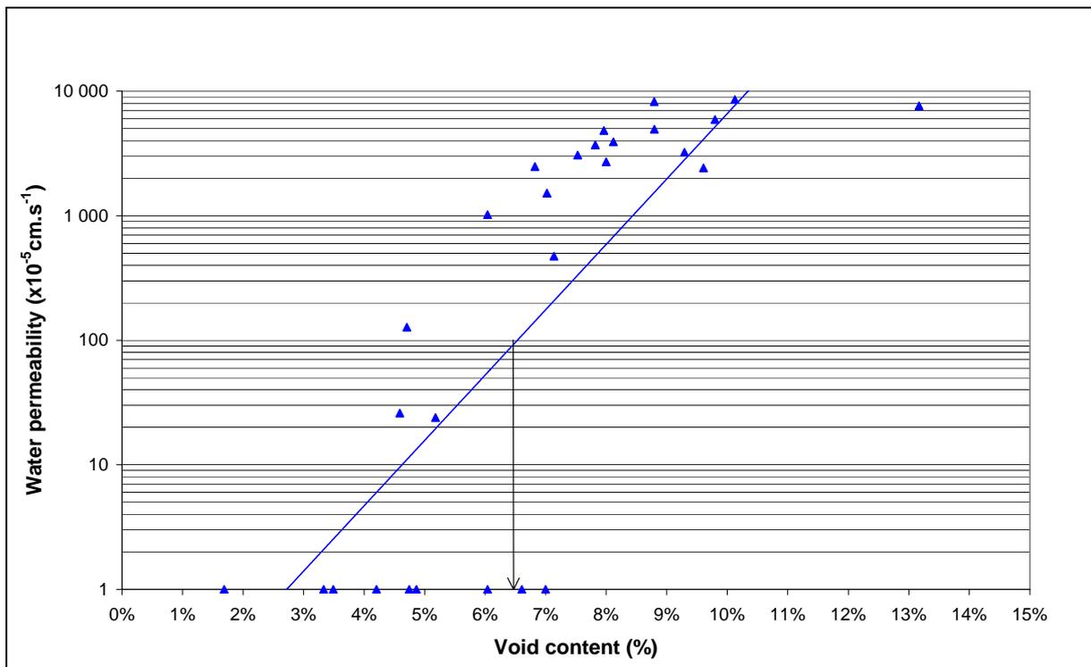
Figure 6. Water permeability vs. air voids (medium continuously graded).
