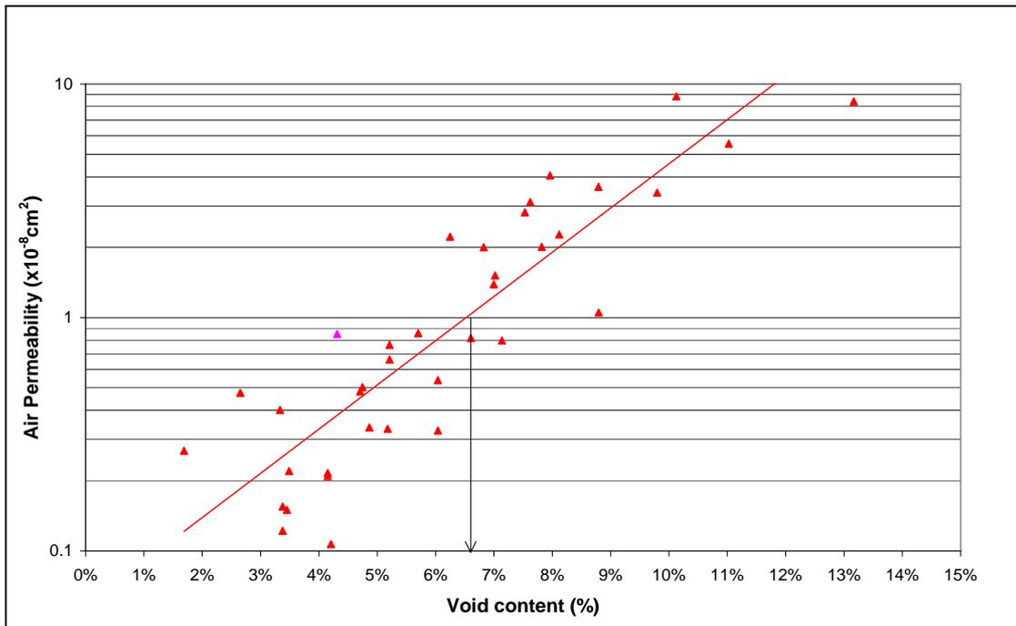
Figure 5. Air permeability vs. air voids (medium continuously graded).
