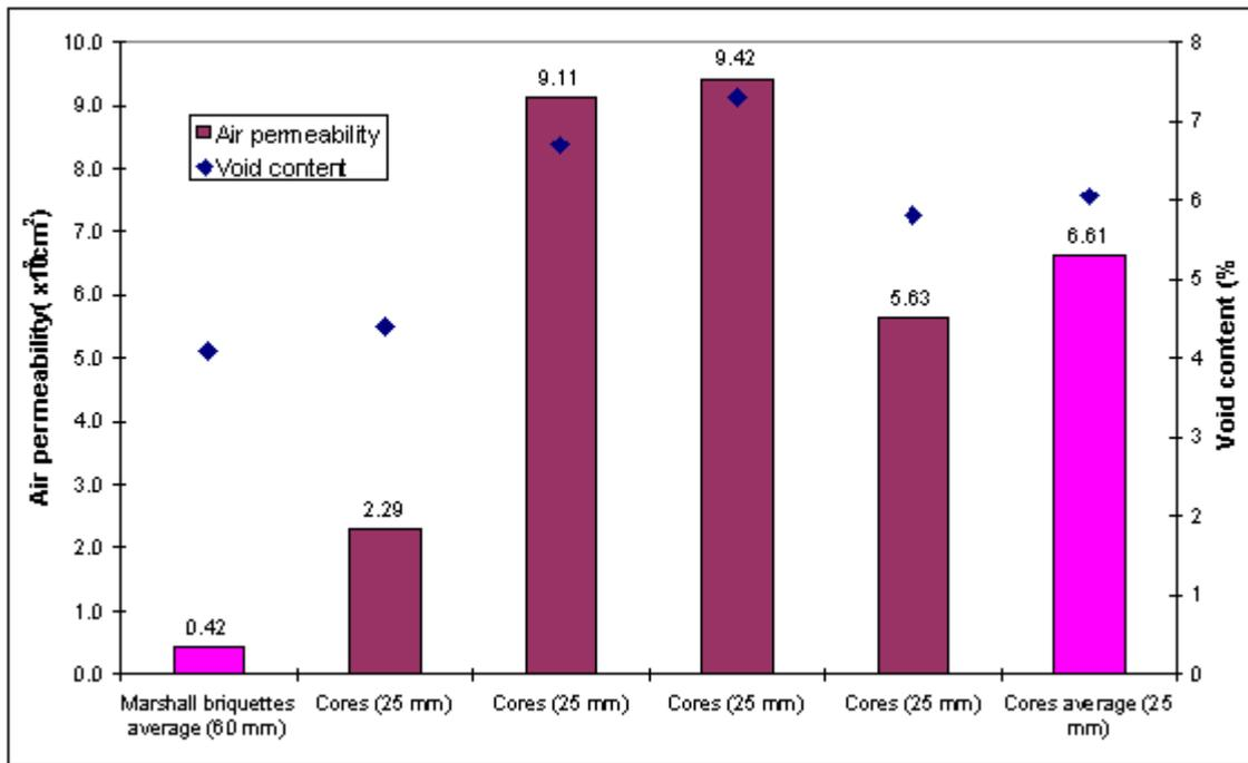
Figure 2. Comparison between laboratory briquettes and core samples (medium continuously graded).
