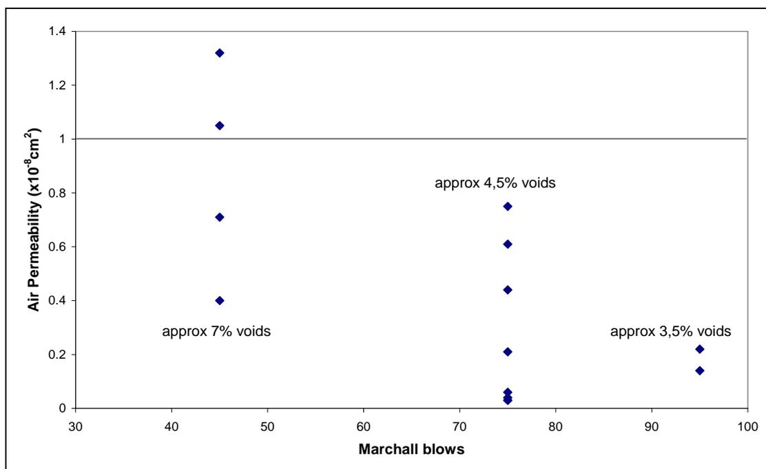
**Figure 1. Comparison between different Marshall compaction levels and air permeability (medium continuously graded).**
